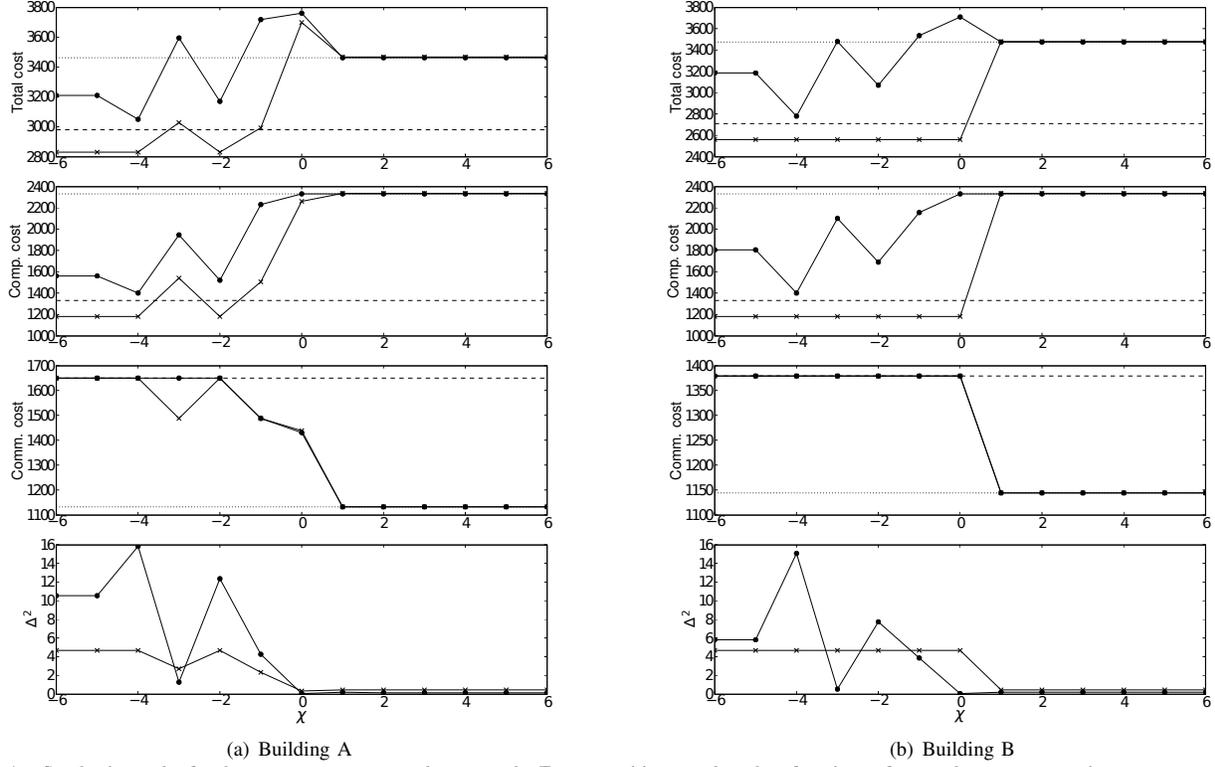
Fig. 4. Synthesis results for the smart-camera network case study. Four quantities are plotted as functions of  $\chi$ : total cost, computation cost, communication cost, and centralization degree  $\Delta^2$ . The horizontal lines correspond to a manual centralized design (dashed) and a manual distributed design (dotted). The two other lines are obtained with *Local Computation Synthesis* (solid lines with dot markers), and *Global Computation Synthesis* (solid lines with star markers).
